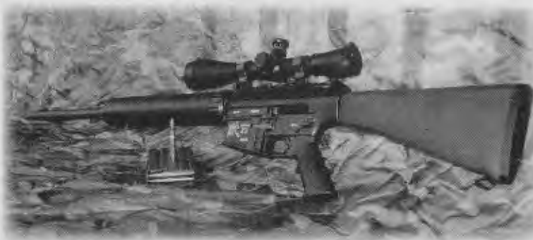
SR-25: Gas-operated, semi-automatic 7.62mm Stoner SR-25 rifle with 20-round detachable box magazine will allow Marine snipers to keep firing at moving targets without having to take their eyes off the enemy while they bolt another round into the chamber. Photo Courtesy of Knights Mfg. Co.
